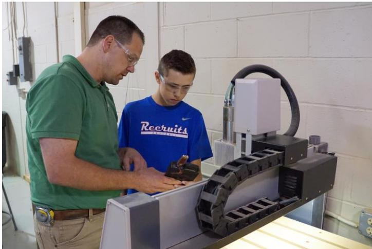
Students begin by creating a computer design that gets converted into coordinates. The cutting spindle on the CNC machine moves to various positions, shapes and depths, as directed by the coding instructions. These processes combine to create two- and three-dimensional patterns out of wood, metal or plastic. The system has practical applications in manufacturing, parts fabrication, milling, engineering, engraving and more.
